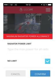
The Smartbox will switch off the radiators with lower priority but also considering the difference between the setting temperatures and measured temperatures to avoid cold zones at the house.
